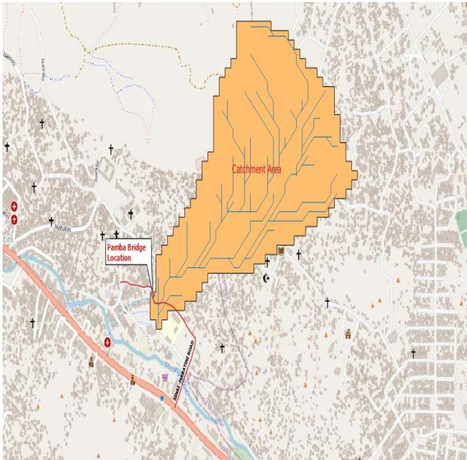
Discharge “Q” was found as **11m<sup>3</sup>/s** and Velocity of flow “V” as **3.4m/s**
